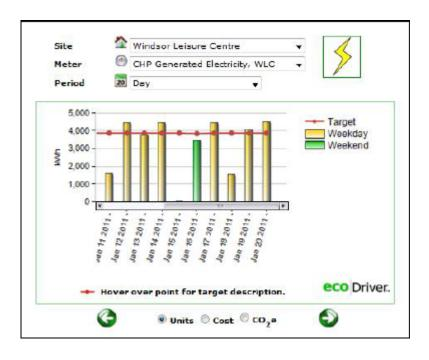
consumption rises. If this is not noticed by the CHP operator then it may be some time before the unit is re-started and consequently the centre may exceed their daily target for grid electricity consumption.
